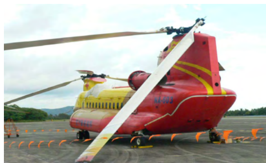
Figure 1 The rear blades' fractured blade damper/shock absorber resulted in the blade's collapse and striking the fuselage
